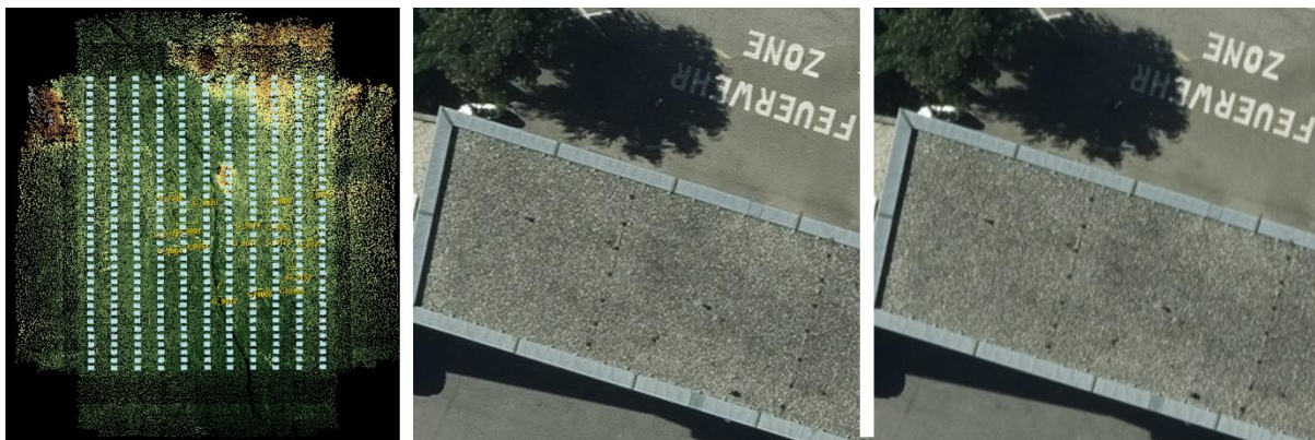
Fig. 7: Flight mission of UltraCam Osprey 4.1, GSD nadir 5 cm, 304 images (cf. left image). Some forward motion blur exists (cf. right image) and was successfully compensated by AMC (cf. central image)
