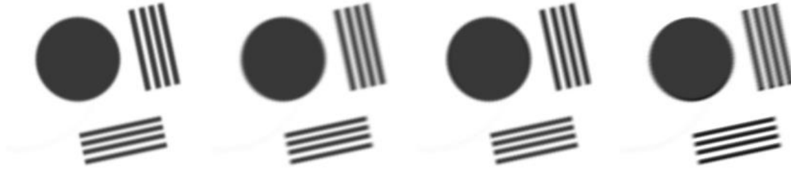
Fig. 4: Illustrating the concept of a deconvolution based on a known PSF. From left to right: original image, blurred image (motion blur at a direction of 20^\circ ), restored image making use of the proper PSF and image processed under wrong PSF parameters (blur direction perpendicular to the blur direction).
