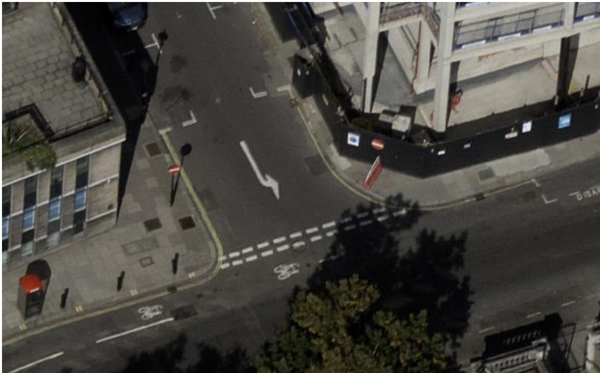
Fig. 2: Oblique backward image of a large-scale flight mission (London, GSD Nadir:3,5 cm). The image has been processed with adaptive motion compensation (AMC) enabled.
