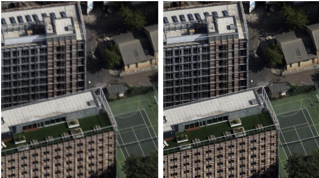
Fig. 6: Details of building facades within a large-scale oblique image (UltraCam Osprey 4.1, GSD nadir 3,5 cm). Strong angular motion blur exists (cf. left image) and was successfully compensated by AMC (cf. right image)
