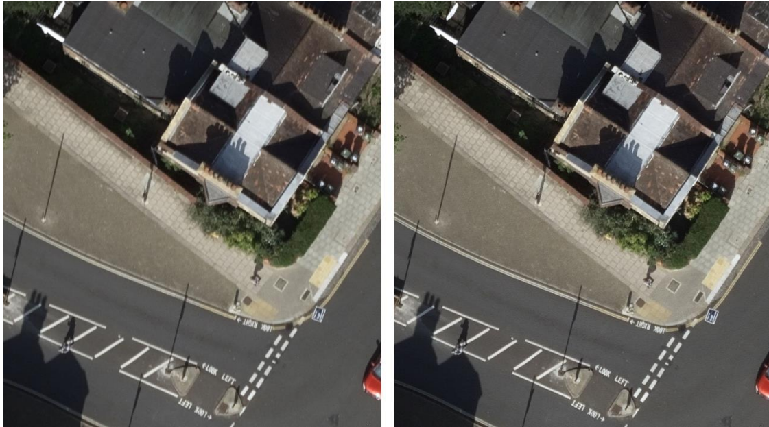
Fig. 5: Street details of one large scale NADIR image (UltraCam Osprey 4.1, GSD nadir 3,5 cm). Motion-blur exist due to suboptimal flight conditions (cf. left image) and was successfully compensated by AMC (cf. right image)
