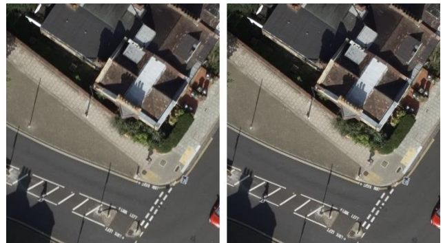
Figure 5: Street details of one large scale NADIR image (UltraCam Osprey 4.1, GSD nadir 3,5 cm). Motion blur exists due to suboptimal flight conditions (cf. left image) and was successfully compensated by AMC (cf. right image)
