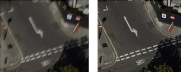
Figure 3b: Street details of one large scale oblique image (cf. Figure 3 a). Strong angular motion blur at about 11 pixel exists in the raw image data (cf. left image) and this was successfully compensated by AMC (cf. right image)
