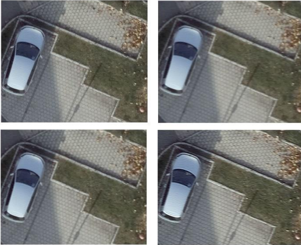
Figure 4: Illustrating the concept of a deconvolution based on a known PSF. From upper left to lower right: original image, blurred image (motion blur at a direction of 20°), restored image making use of the proper PSF (lower left) and the image processed by incorrect parameters.
