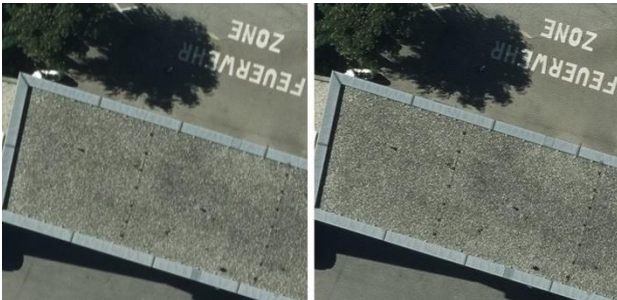
Figure 8: Some forward motion blur exists (cf. left image) and was successfully compensated by AMC (cf. right image)
